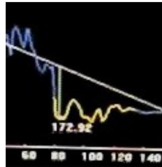
Figure 2: Automatic location of a stenosis in a user-chosen segment of artery with Philips' "Computer-Assisted Aneurysm Analysis" package for their *Allura* 3D-RA, in use at a local hospital. The curve shows actual diameter (in mm) between the endpoints. The section of curve in yellow indicates the stenosis. The point of greatest deviation is marked. Location of aneurysms is analogous.
