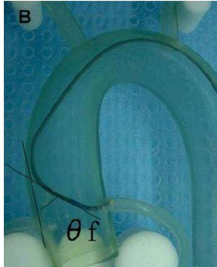
(b) The JL4 as deployed [Ikari 2005]. Notice that catheters do not follow the midlines of arteries, as most computer simulations would have it.
